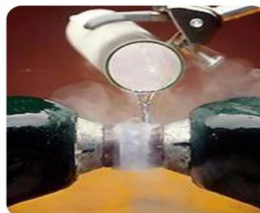
Liquid oxygen is attracted and gets suspended between the poles of a strong magnet
